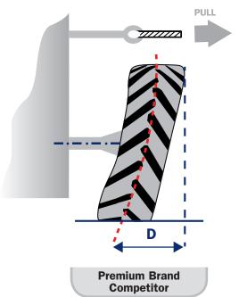
Test conditions Reference size: 460/70R24 Pull force: from 1,000 Kg to 6,000 Kg D: Displacement
