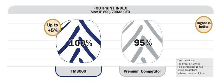
The larger contact area of the TM3000 significantly reduces soil compaction. The wide footprint area provides better flotation
